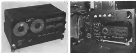
APN-66 PANEL SHOWS heading position, ground speed, wind direction and direction. Device gives pilot steering data to destination.
